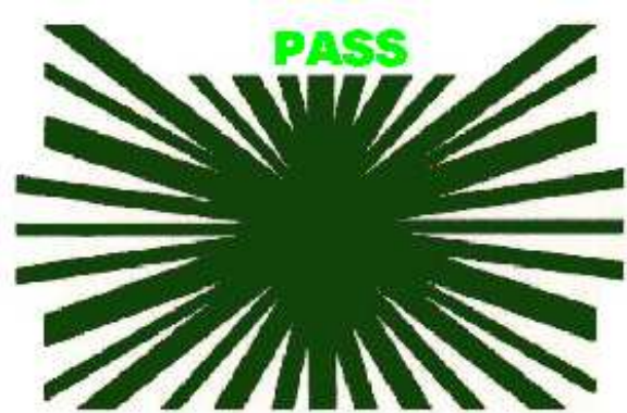
Fig.10 : Test Bowie Dick conforme
